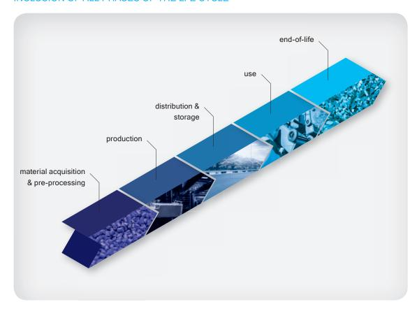
The figures yielded by the assessment showed that the most significant emissions occur in the phases of material procurement and pre-processing (63 % 2-wheel or 68 % 4-wheel) and disposal (25 % 2-wheel or 20 % 4-wheel). The zone directly controlled by us, production, is responsible for less than 1 % of the total emissions. A decisive reason for this is that we use green energy only. In the total carbon footprint of a bin, this leads to
